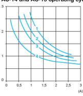
AC-14 Control of weak electromagnetic loads of electromagnets  $\leq$  72 VA (make:  $\cos \varphi = 0.3$ , break:  $\cos \varphi = 0.3$ )
